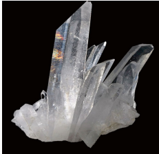
Figure 1: Quartz Crystal - Quartz is a simple crystal structure comprised of silicon-oxygen tetrahedral, \text{SiO}_4 [2].
