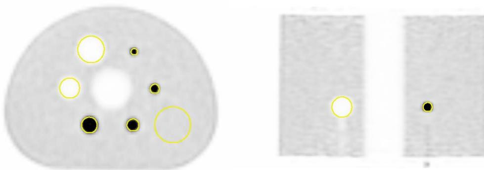
Figure 6. The phantom image showing the volumes of interest used in the analysis.
