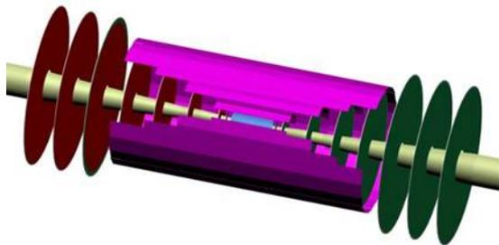
Fig. 1. Intermediate tracker (IMT) at Global Large Detector (GLD) concept in the international linear collider and the silicon vertex detector inside the IMT is shown in blue color. The barrel and endcap of the IMT consist of 4 and 7 layers of silicon detector.
