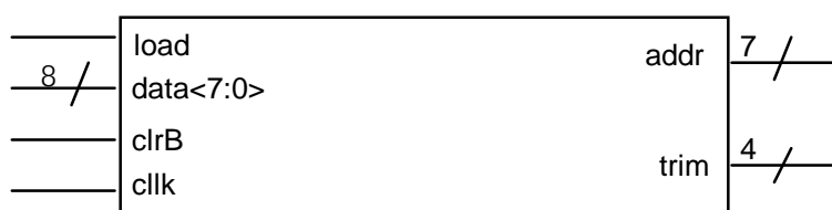
Figure 3.13A. Trim DAC Register Inputs/Outputs.
