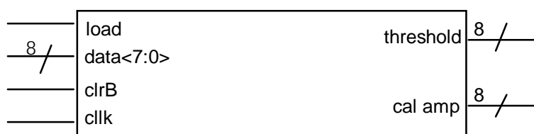
Figure 3.12. Threshold/Calibration DAC Register Inputs/Outputs.
