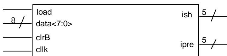
Figure 3.13. Bias DAC Register Inputs/Outputs.
