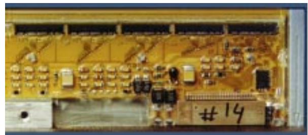
Figure 3.1.4. Photograph of the right-most 1/5 of a hybrid, shown mounted on the side of a BTEM tray.
