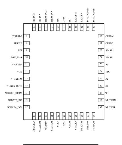
Bonding Pad Layout for the GTRC Chip (not to scale)
