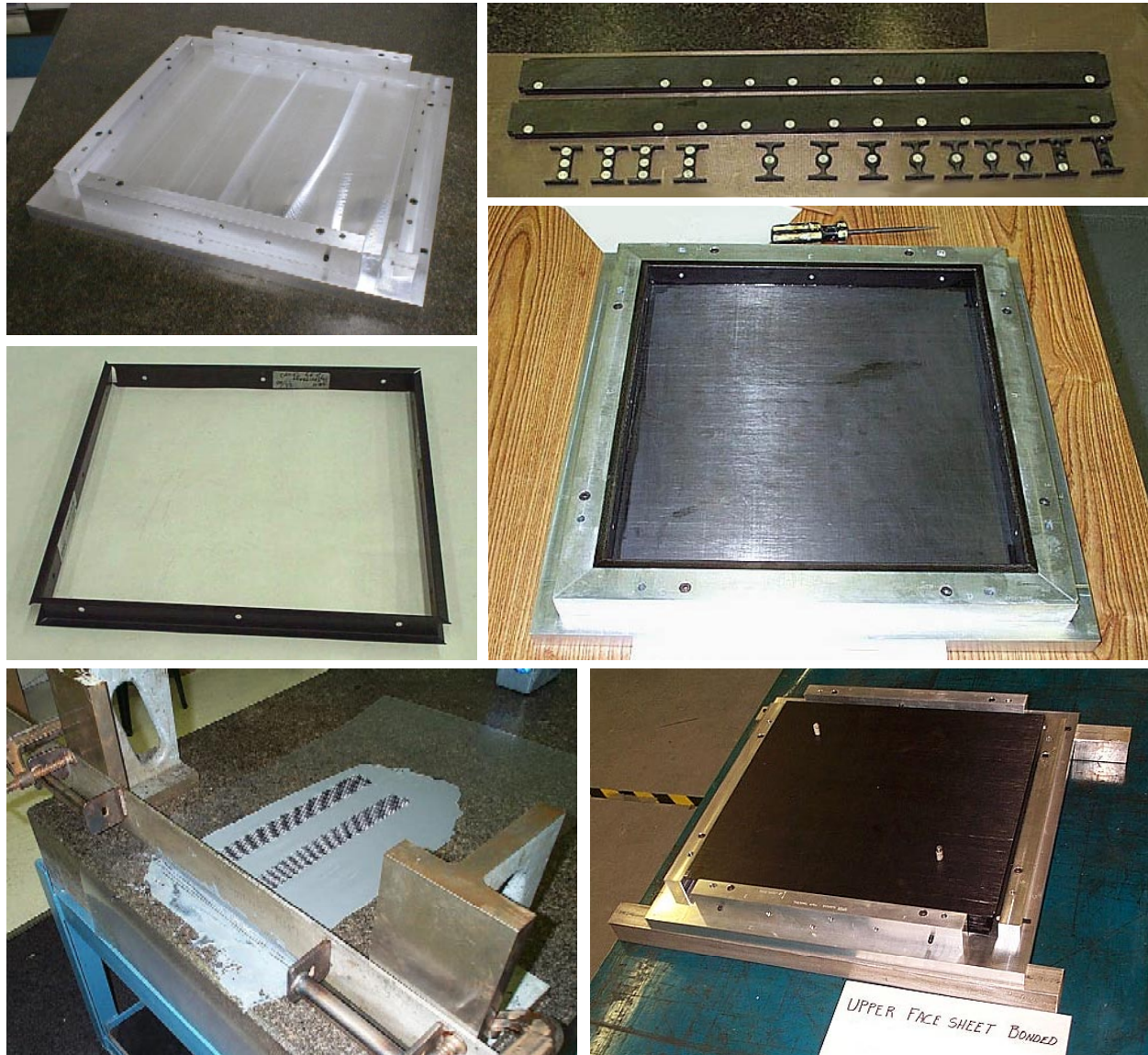
Figure 23: Various assembly steps of Concept 1 composite tray prototype; left to right and top to bottom: the bonding fixture with locating features for thermal sides and brackets, bonding metal inserts into thermal sides and brackets, the 4 'C' channels ready to bond, bonding the 'C' channels to the bottom face sheet, dipping the side cores to minimize the amount of glue, bonding brackets and thermal walls into 'C' channels.
