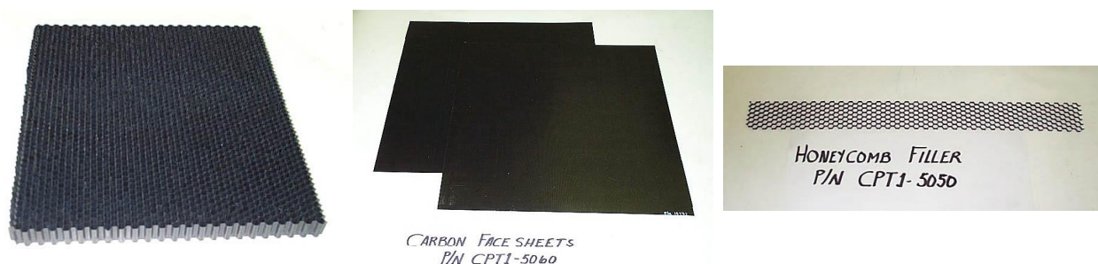
Figure 20: Left to right: main GFRP honeycomb core, GFRP face sheets, and side/filler core.
