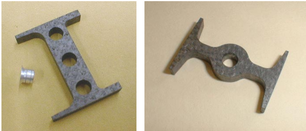
Figure 22: corner (left) and center (right) clips used for concept 1 tray prototype; the parts were made of 2D CC; left view also shows one of the metal inserts to be bonded and later drilled and threaded.
