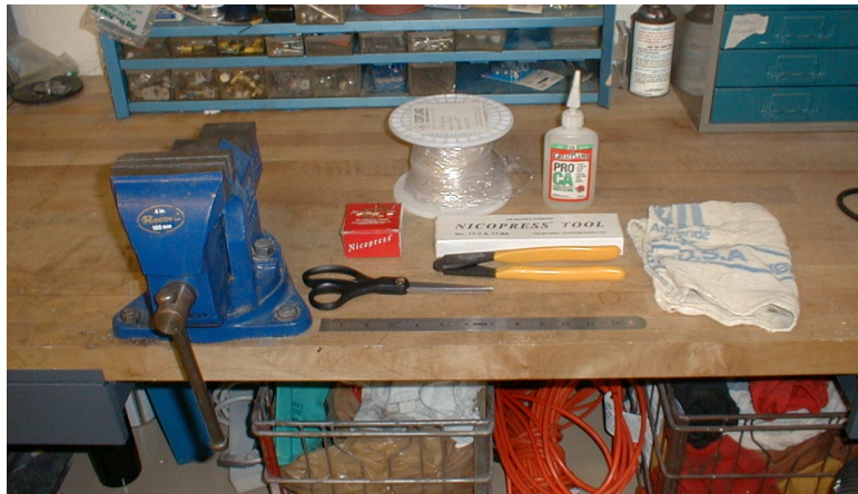
Figure 2: Supplies for cable termination.
