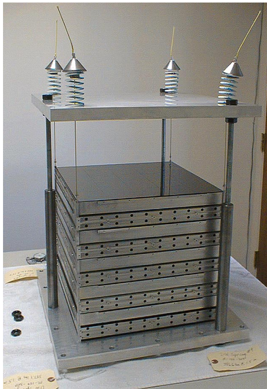
Figure 7: NASA SBIR Phase I tower in tensioning fixture.
