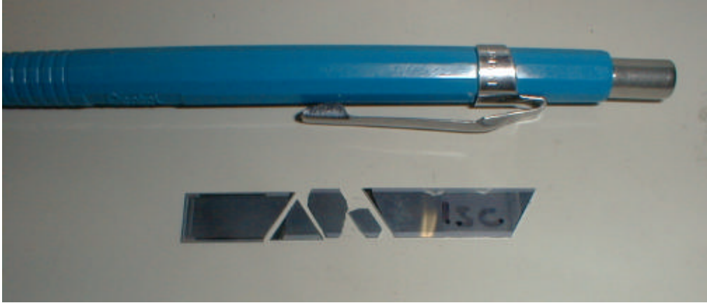
Figure 4: Baby sample 1s-c after bend test
