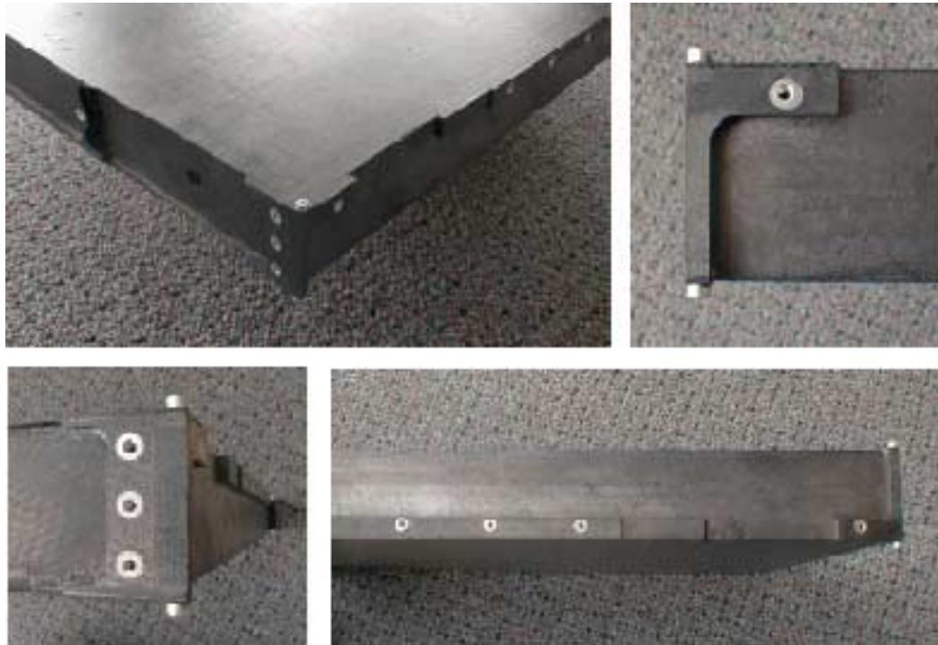
Figure 2.1.1. Photographs of the Hytec carbon-fiber tray prototype, constructed with SBIR funding.
