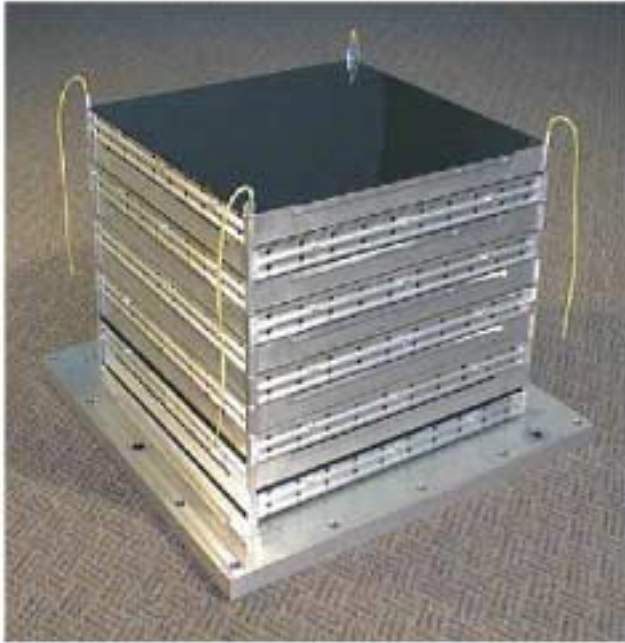
Figure 2.1.2. The aluminum-closeout tower built by Hytec with NASA SBIR funds to validate the GLAST structural design concept.
