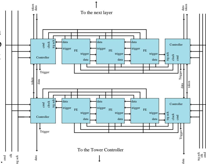
*Simplified block diagram of the readout of a GLAST tower, showing only 2 of 16 layers and only 3 of 25 readout chips on each layer.*
