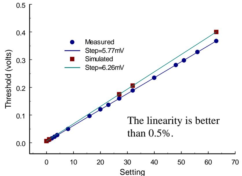
*Measurement of the DAC performance in the low range, compared with a Spice simulation of the circuit. The slope is close to expectations despite the error in the resistor values.*
