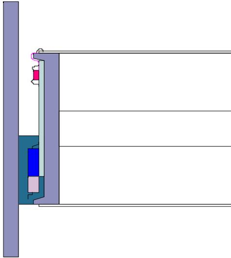
To minimize dead area, the hybrid circuits holding the readout chips and controller chips must be mounted on the sides of the detector trays.
