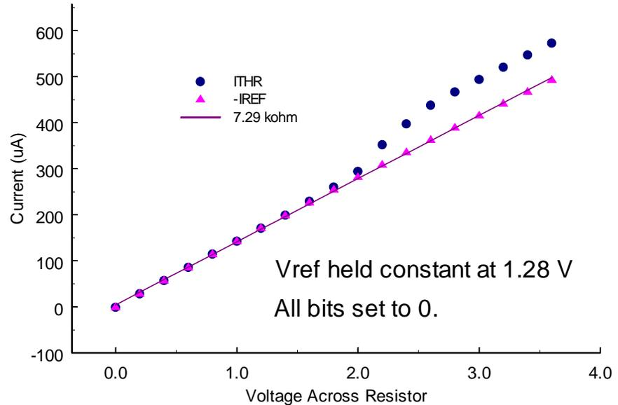
*With V-ref held constant, V-threshold is scanned from V-ref up to 5 V. Above a certain point there is more current flowing into the threshold node than is flowing out the opposite end of the resistor.*
