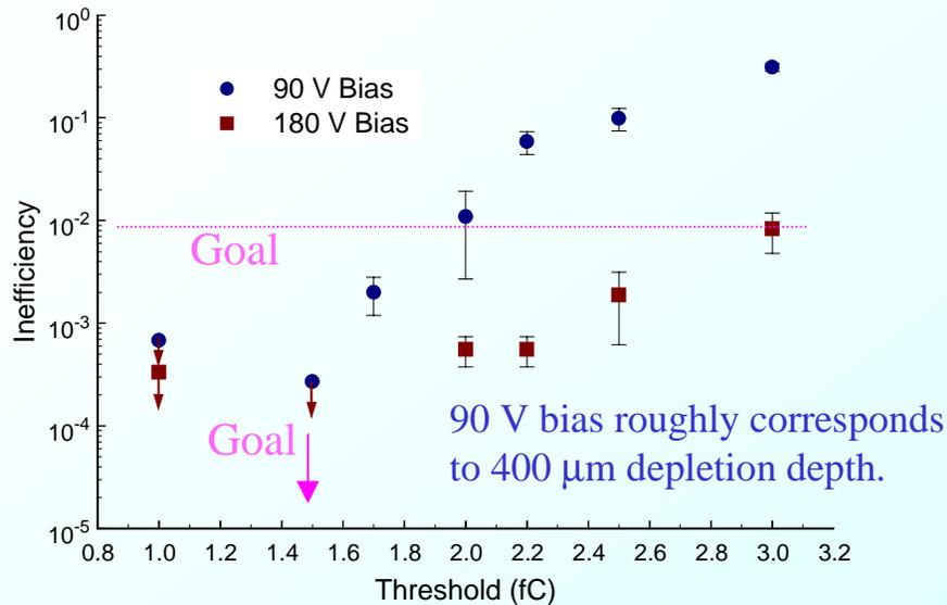
*Inefficiency for detection of minimum ionizing electrons at normal incidence in a single detector plane.*
