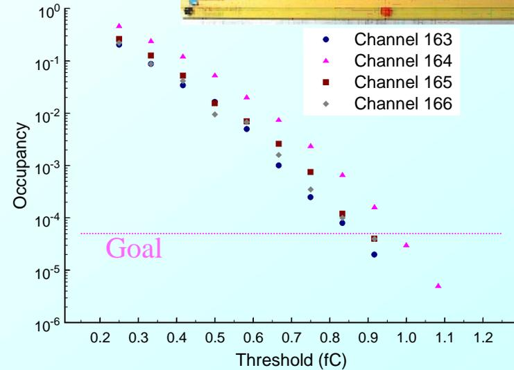
*Noise occupancy, in a 1  $\mu\text{s}$  window, versus threshold for four different channels connected to 30 cm long detector strips.*
