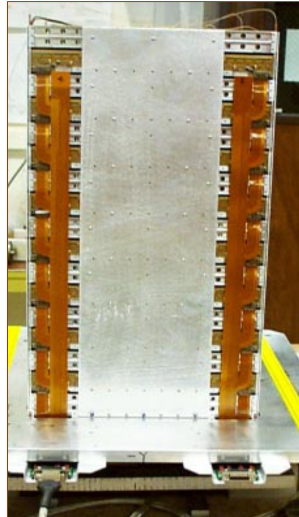
The completed beam-test tracker, with 2 side panels removed.
