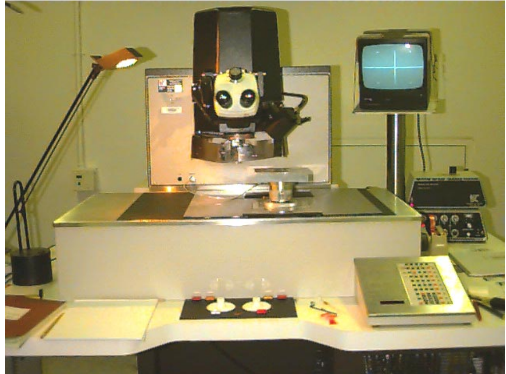
The large-area automated wire bonder at UCSC.
