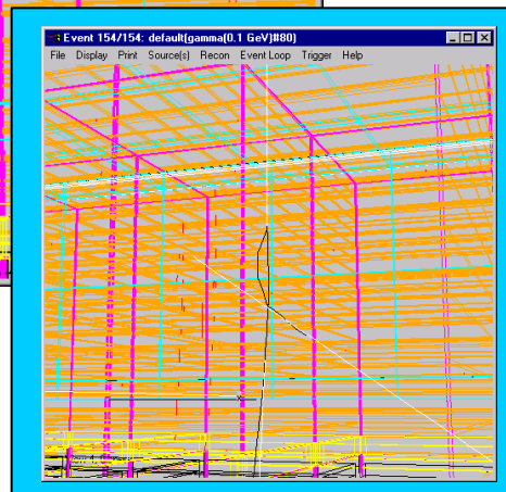
A gamma event reconstructed in 3D using the Pair Fit
