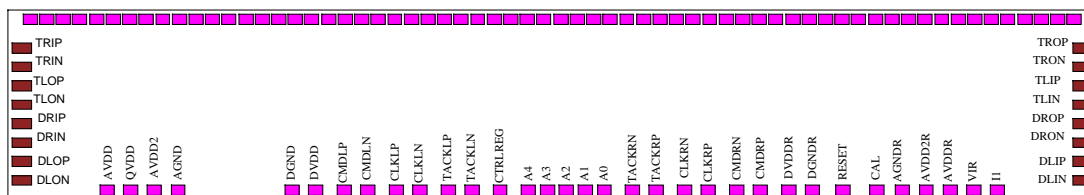
Figure 1. Bonding pad layout of the GTFE64B chip (not to scale). Channel 0 is on the left.
