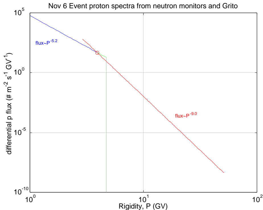
Fig. 8 - Calculated differential flux of isotropic protons from the 6 November 1997 SEP event. Below \sim 4 GV, the neutron monitor derived flux spectrum is shown. Above \sim 4 GV, two possible spectra that are consistent with the Milagrito high threshold scaler rate increase are shown. One of these spectra involves a hard cutoff of the spectrum from lower energies, while the other curve is a broken power law. The actual spectrum is probably a gradual rollover of the rigidity power law. The circle is placed at the point where the neutron monitor and the Milagrito derived spectra were required to overlap.
