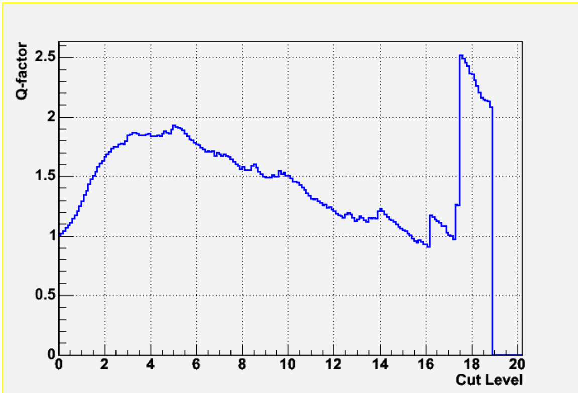
Figure 8 Q-factor as a function of the cut level. Events with n_{\text{Top}}/c_{\text{xPE}} less than the cut level are excluded.
