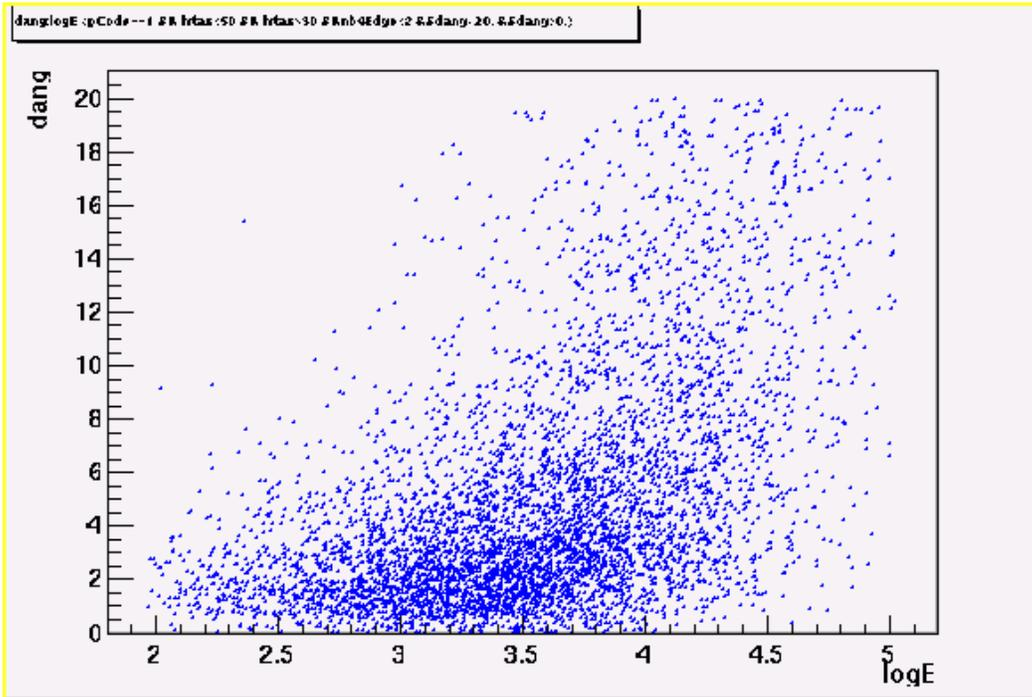
Figure 19 Angle error vs. primary energy for events with  $30 < n_{Top} < 50$ .
