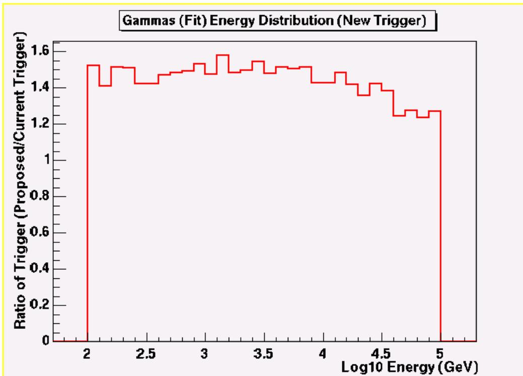
Figure 11 Ratio of the two curves in Figure 10. On average the new trigger increases the effective area for gamma rays by 45%.
