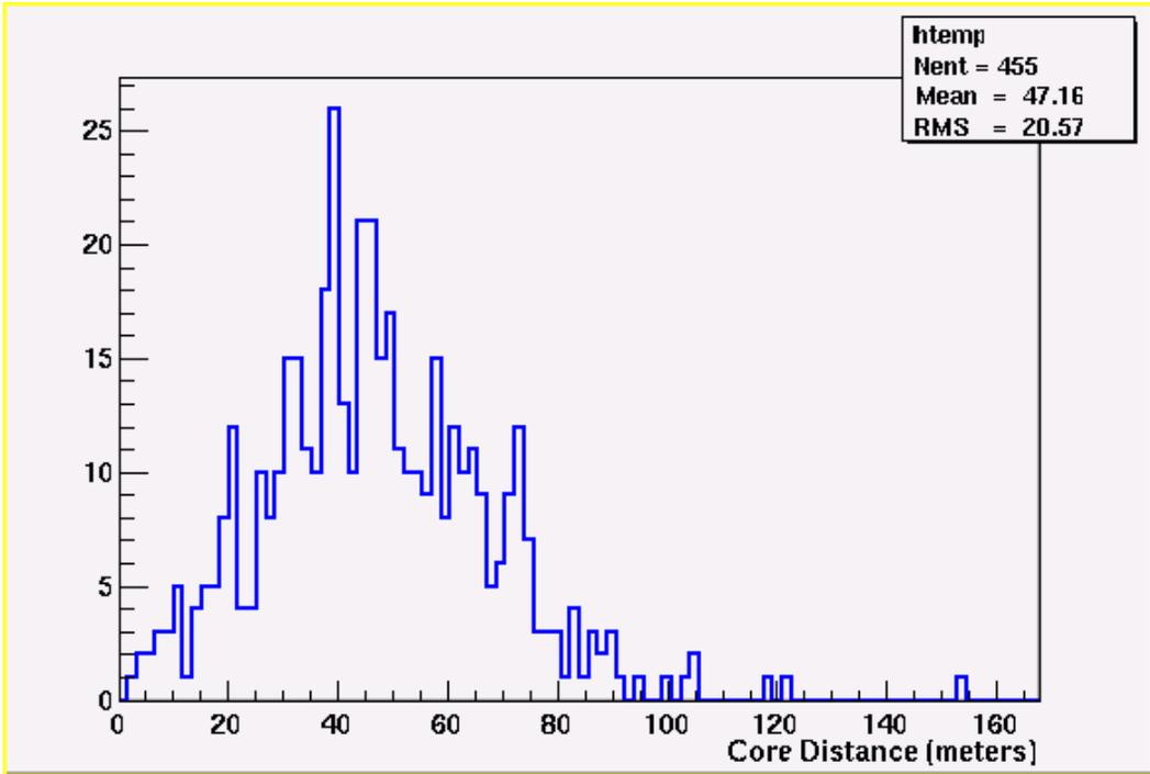
Figure 16 Core distance distribution for new events ( $n_{\text{Top}} < 50$ ) with primary energy less than 500 GeV.
