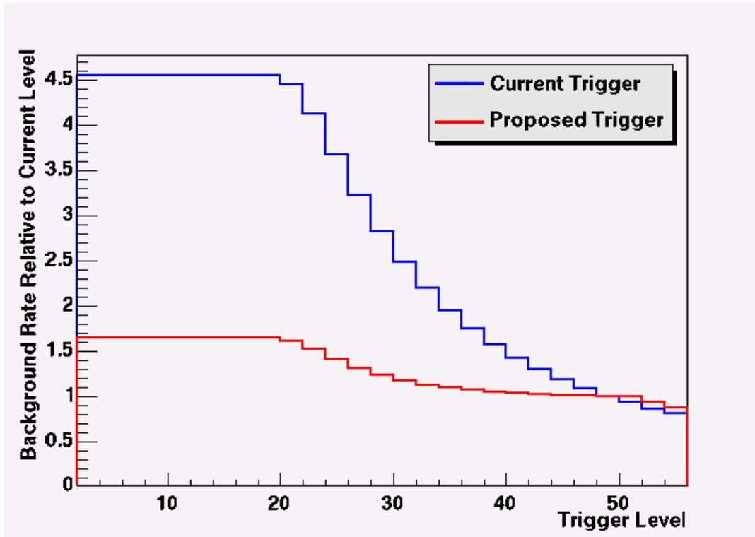
Figure 12 Relative (to current level) increase in fit background as a function of nTop.
