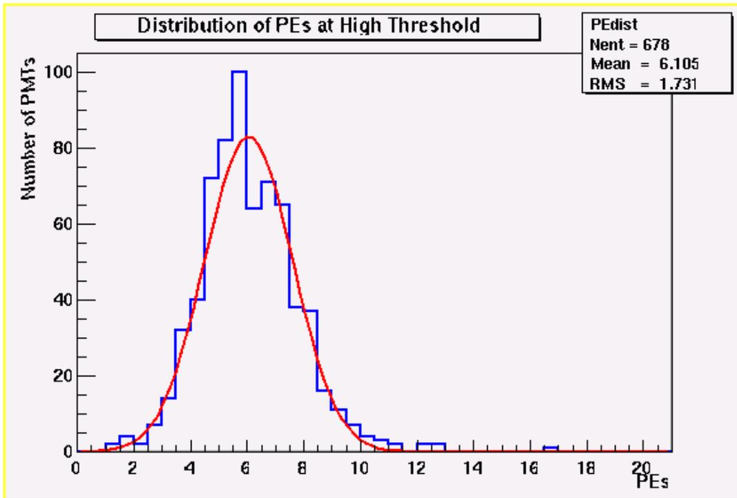
Figure 5 Measured values of high threshold (in PEs) for all PMTs in the pond. The red line is a Gaussian fit to this distribution.
