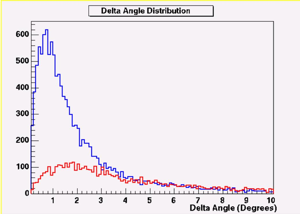
Figure 13 *delAngle* distribution of current events (blue) and new events (red). *delAngle* is the space angle difference between the true direction and the reconstructed direction.
