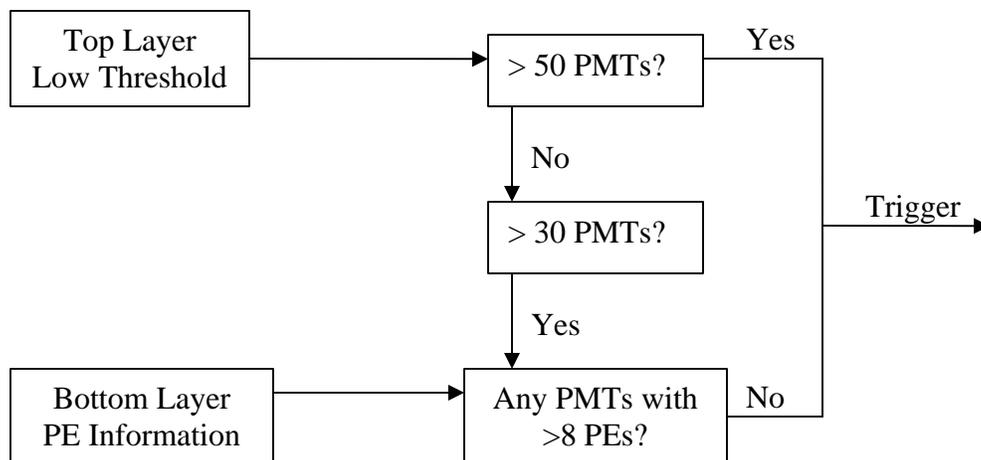
**Figure 1 Old Proposed Intelligent Trigger**
