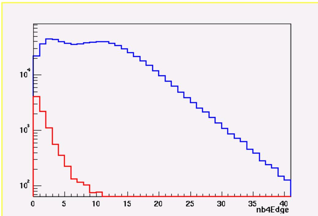
Figure 6 Distribution of number of 4-Edge PMTs for events with  $30 < n_{\text{Top}} < 50$ . Blue line is data, red line is gamma Monte Carlo.
