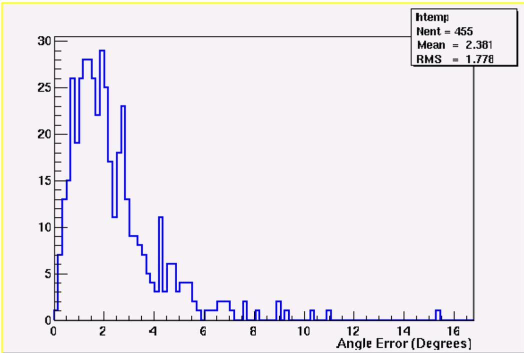
Figure 17  $\Delta\theta$  distribution for new events ( $n_{\text{Top}} < 50$ ) with primary energy less than 500 GeV.
