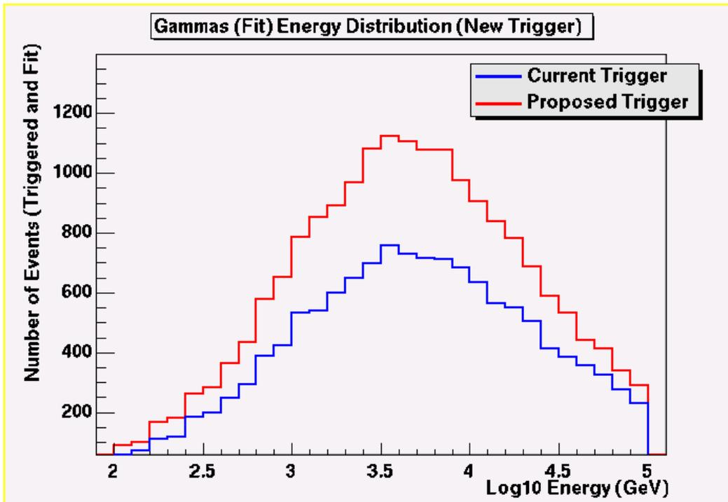
Figure 10 Number of triggers as a function of energy for the current trigger and the proposed trigger. The gamma rays were thrown on an  $E^{-2.4}$  spectrum.
