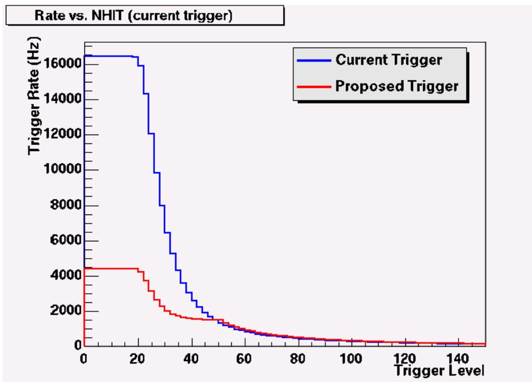
Figure 8 Trigger rate as a function of nTop for the current trigger (blue) and the propose trigger (red).
