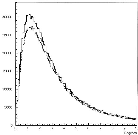
Fig. 17. The distribution of  $\Delta_{EO}$  for events with  $N_{Fit} \geq 40$  for the three different water depths. The dashed histogram is for 1 m, the solid is for 1.5 m, and the dotted is for 2 m. Note that the three histograms are normalized to have the same areas.
