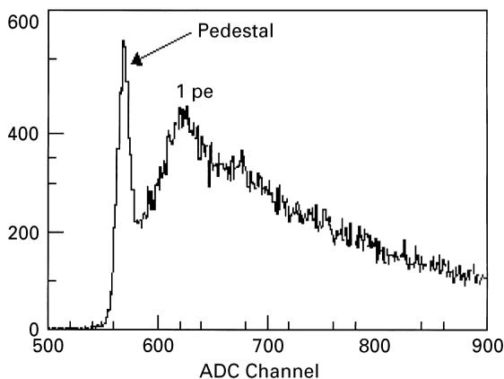
Fig. 5. The measured ADC spectrum for a typical Hamamatsu R5912SEL photomultiplier showing the ADC pedestal (channel  $\sim 570$ ) and the single PE peak (channel  $\sim 625$ ). The conversion to charge is 50 fC/channel.
