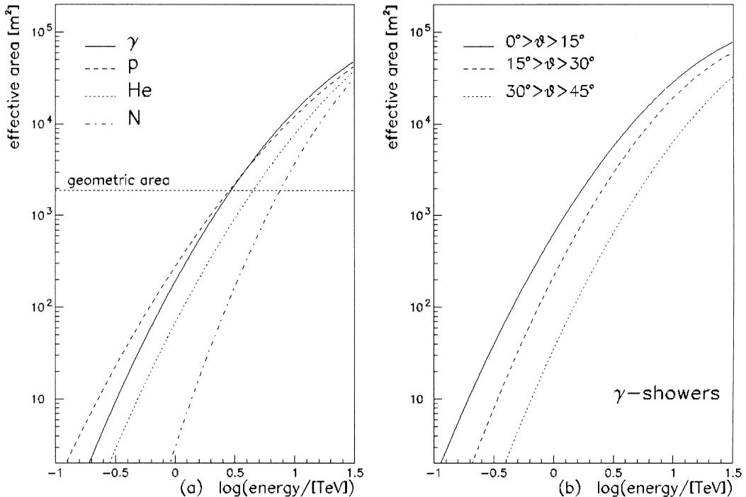
Fig. 20. (a) The effective area,  $A_{\text{eff}}$ , as a function of the energy of the primary particle for hadron and photon showers; (b) The dependence of  $A_{\text{eff}}$  with zenith angle for photon showers.
