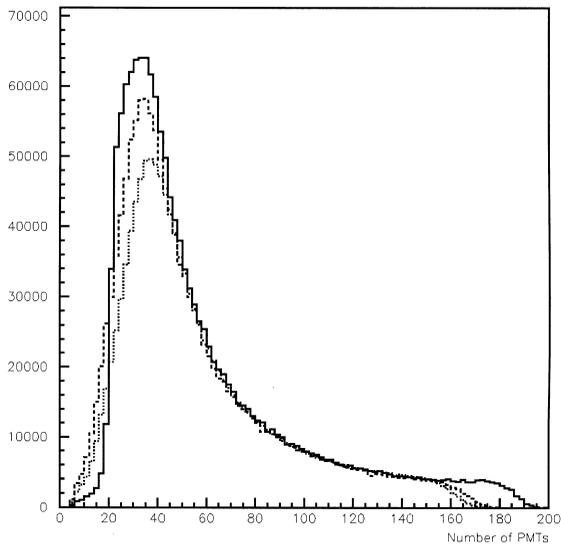
Fig. 16. The distribution of the number of events versus  $N_{Fit}$  for water depths of 1 m (solid histogram), 1.5 m of water (dashed histogram), and 2 m of water (dotted histogram). The three histograms are normalized to have the same areas. Note that the number of working PMTs is higher for the 1-m data.
