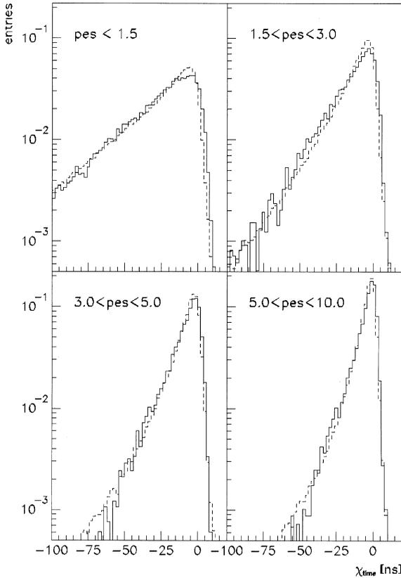
Fig. 13. The difference between the shower plane and the measured PMT time,  $\chi_t$ , for PMTs with the number of detected photoelectrons in the ranges 0–1.5, 1.5–3, 3–5, and 5–10, for experimental data (dotted line) and simulated data (solid line). Note that  $\chi_t$  increases as the PMT time gets earlier.
