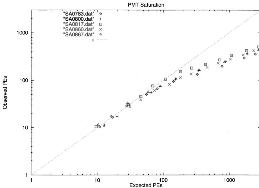
Fig. 6. The observed number of photoelectrons versus the expected number for 5 Hamamatsu R5912SEL photomultipliers as measured with a pulsed laser and attenuating filters.
