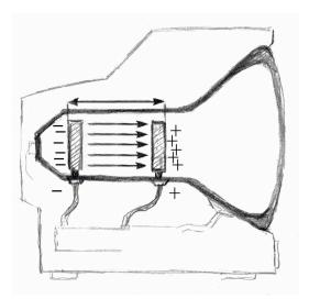
22. Collisions of electrons with the surface of your television set give rise to the images you see. How are the electrons accelerated to high speed? Consider the following: two metal plates (The right hand one has small holes allow electrons to pass through to the surface of the screen.), separated by 30 cm, have a uniform electric field between them of 400 N/C.
