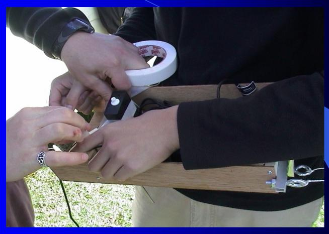
2. Hooked up equipment to gondola: LabPro to record data, pressure probe to measure atmospheric pressure, and thermometer to measure air temperature.
