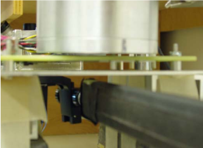
Close up of the spatial relationship between the scintillator and SSD module.
