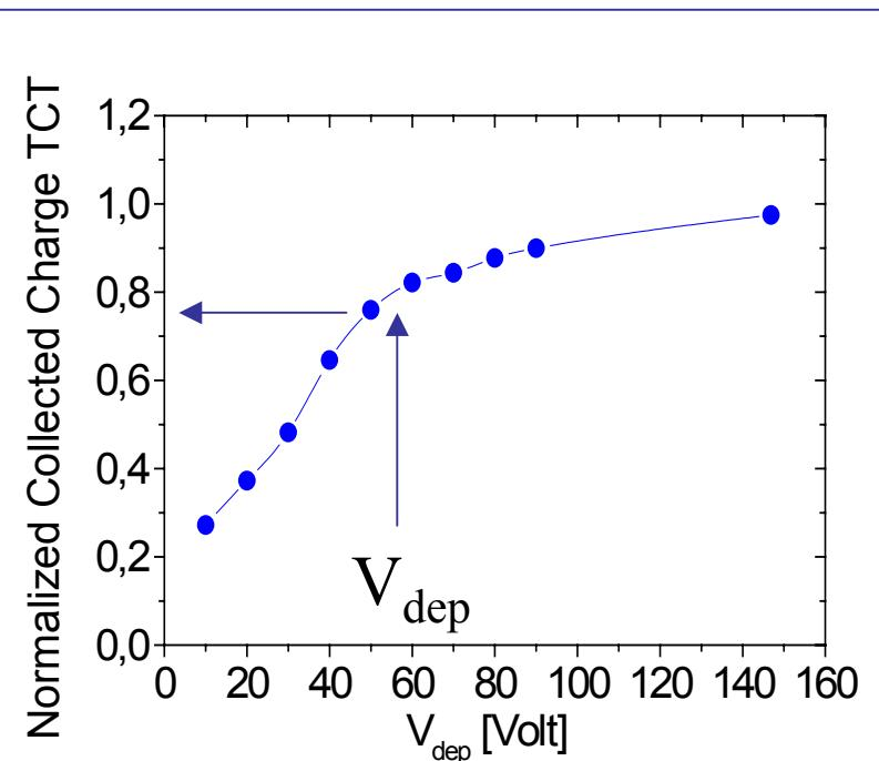
To maximise CCE it is necessary to overdeplete the detector up to :
