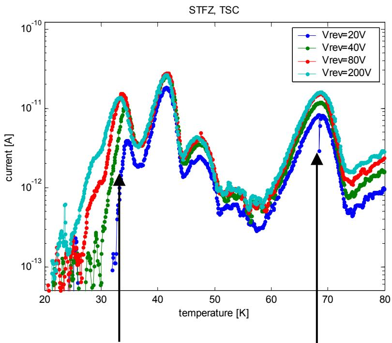
26 MeV p irradiated,  $\Phi=2.5\times10^{14}$  n/cm<sup>2</sup>
