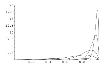
As  $N \to \infty$ ,  $F_N(x) \to 0$  but in a very non-uniform way, since the area under the graph of  $F_N(x)$  approaches 1 in the same limit!
