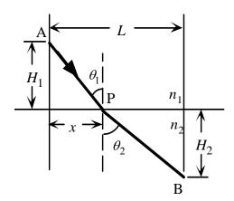
$$t_{AB} = t_{AP} + t_{PB} = \left[ (x^2 + H_1^2)^{1/2} / (c/n_1) \right] + \left\{ \left[ (L - x)^2 + H_2^2 \right]^{1/2} / (c/n_2) \right\}.$$
