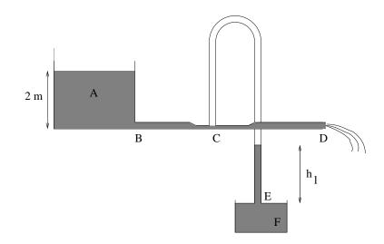
b) The pipe BCD is now sealed off at D. Water rises at C, and falls at E. We wait till all the water stops flowing. Assume that the gas trapped inside the curved tube CE is incompressible. The tube is of uniform cross section. What is the height of water at C and E,  $h_2$  and  $h_3$  respectively?
