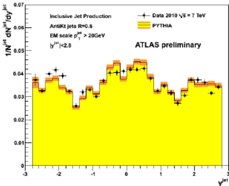
Observed jets with  $PT > 20\text{ GeV}$  using MinBias trigger and integrated luminosity  $\sim 350\ \mu\text{b}^{-1}$
