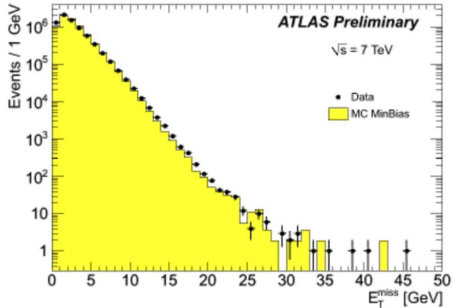
Missing  $E_T$  computed using noise-suppressed clusters at EM scale, integrated luminosity  $\sim 110 \mu\text{b}^{-1}$
