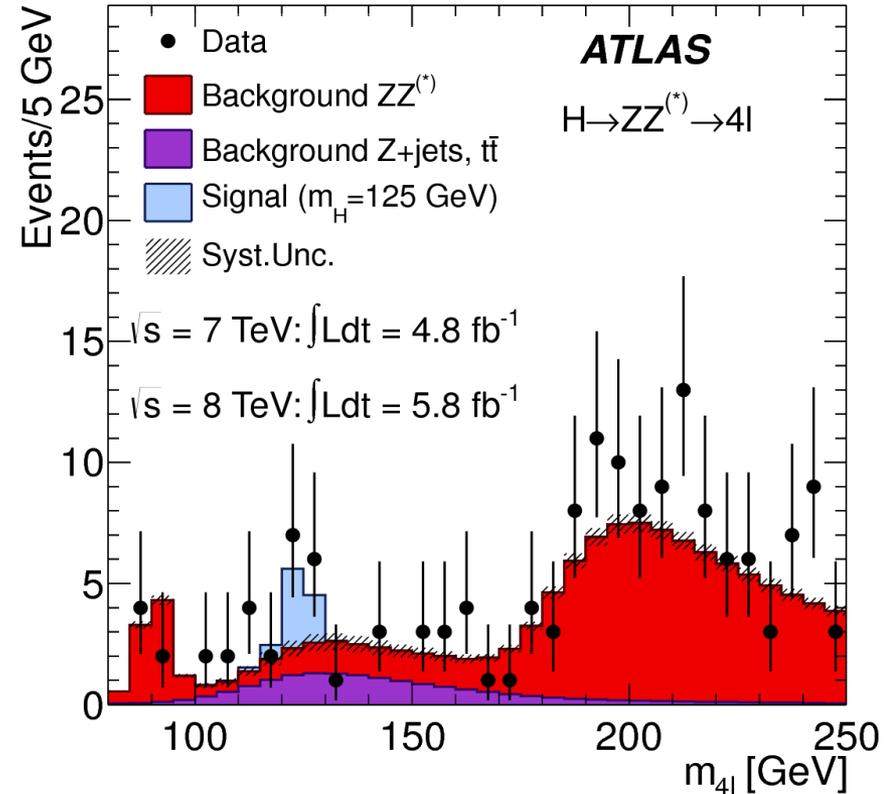
The distribution of the four-lepton invariant mass,  $m_{4l}$ , for the selected candidates, compared to the background expectation in the 80 to 250 GeV mass range, for the combination of the 7 TeV 8 TeV data. The signal expectation for a Higgs boson with  $m_H = 125$  GeV is also shown.
