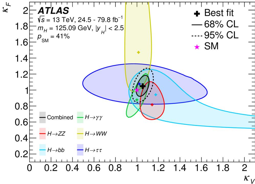
Negative log-likelihood contours at 68% and 95% CL in the  $(\kappa_F, \kappa_V)$  plane for the individual decay channels and the combined fit, assuming that the coupling strengths to fermions and vector bosons to be positive. No contributions from invisible or undetected Higgs boson decays are assumed. The best-fit value for each measurement is indicated by a cross while the SM hypothesis is indicated by a star. Taken from ATLAS collaboration, Phys. Rev. D 101, 012002 (2020).
