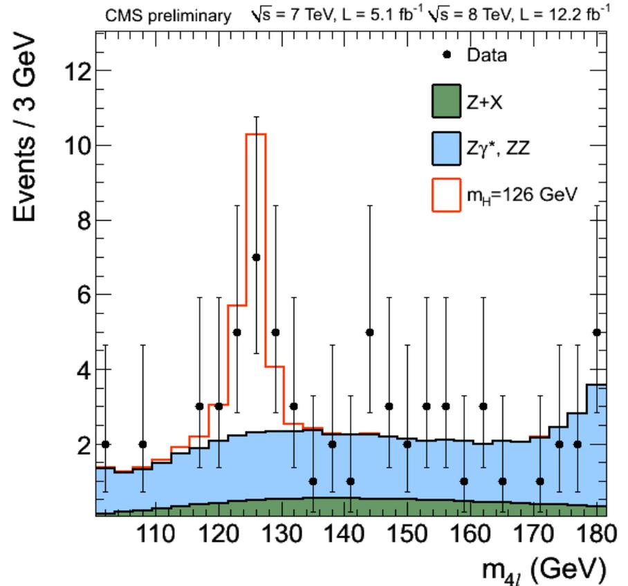
Distribution of the four-lepton invariant mass for the  $ZZ \rightarrow 4$  leptons analysis. The points represent the data, the filled histograms represent the background, and the open histogram shows the signal expectation for a Higgs boson of mass  $m_H = 126 \text{ GeV}$ , added to the background expectation. Taken from <https://twiki.cern.ch/twiki/bin/view/CMSPublic/Hig12041TWiki>.
