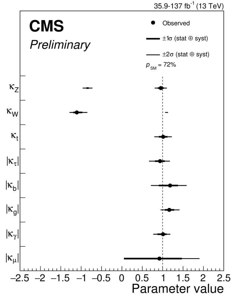
Summary of the  $\kappa$  framework model assuming that there are no additional BSM contributions to the Higgs boson width, i.e.  $\text{BR}_{\text{BSM}} = 0$ . The points indicate the best fit values while the thick and thin horizontal bars show the  $1\sigma$  and  $2\sigma$  CL intervals, respectively. Taken from CMS Collaboration, CMS-PAS-HIG-19-005 (January, 2020).
