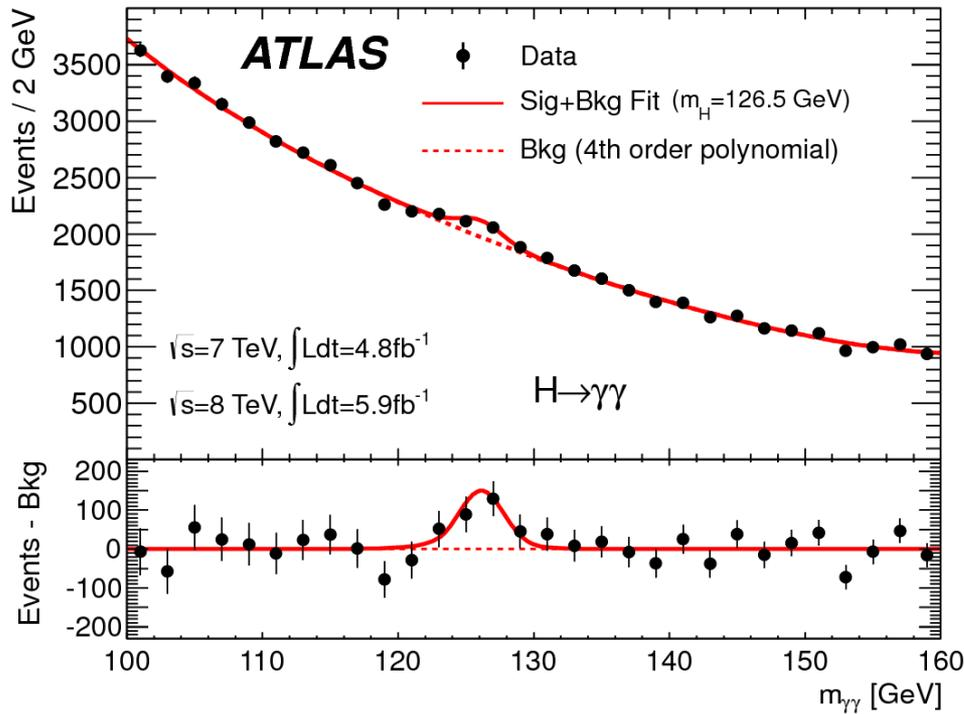
Invariant mass distribution of diphoton candidates for the combined 7 TeV and 8 TeV data samples. The result of a fit to the data of the sum of a signal component fixed to  $m_H = 126.5$  GeV and a background component described by a fourth-order Bernstein polynomial is superimposed. The bottom inset displays the residuals of the data with respect to the fitted background component.
