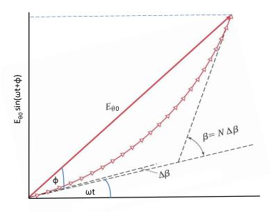
Note that  $\Delta E_0$  is the length of each of the N phasors in the above figure. We can apply the limit of  $N\to\infty$  and  $\Delta y\to 0$  (with  $N\Delta y=D$  held fixed) directly to the phasor diagram above. In this limit, the phasors follow the arc of a circle of radius r whose center is located at C. The arc length from the origin O to the point B shown in the figure below is then  $N\Delta E_0=E_0$ .
