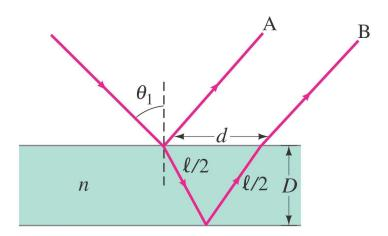
Ray A reflects directly back into the air, while ray B travels a total distance  $\ell$  within the slab before re-emerging from the slab's face a distance d from its point of entry.
