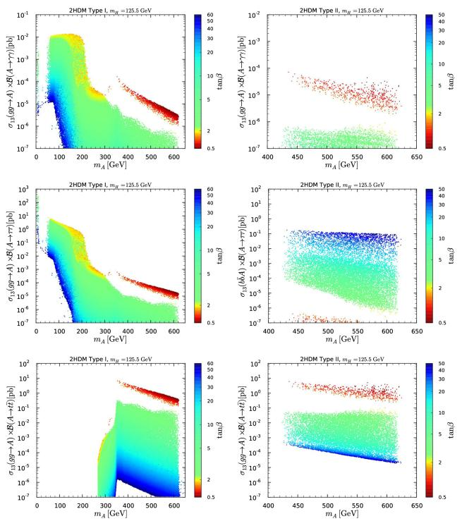
FIG. 18. Cross sections times branching ratios in type I (left) and in type II (right) for  $A \rightarrow Y$  signatures at the 13 TeV LHC as functions of  $m_A$  with  $Y = \gamma\gamma$  (upper panels),  $Y = \tau\tau$  (middle panels) and  $Y = t\bar{t}$  (lower panels) with  $\tan\beta$  color code. Points are ordered from high to low  $\tan\beta$ .
