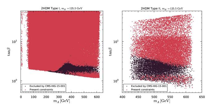
FIG. 20. Projection of the scan points in the plane  $\tan \beta$  vs  $m_A$ , on the left for type I, on the right for type II. The red points are consistent with all constraints used in this paper, while the underlying black points are those which are excluded by the CMS  $A \rightarrow Zh$   $(Z \rightarrow \ell\ell, h \rightarrow b\bar{b}, \tau\tau)$  limit [17] after all other constraints have been applied.
