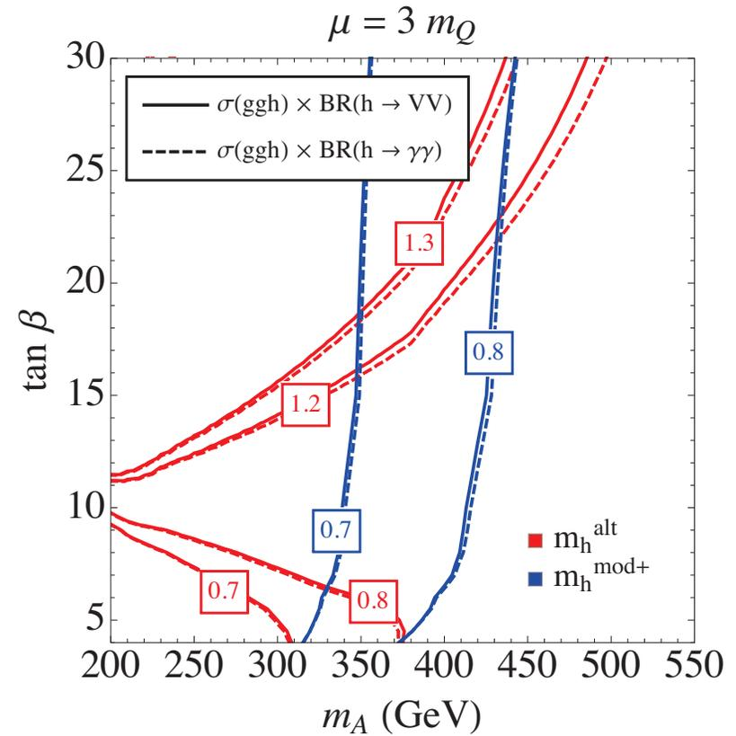
The observed  $h$  is SM-like, albeit with somewhat large errors. If the  $\sigma \times \text{BR}$  for  $h \rightarrow VV$  and  $h \rightarrow \gamma\gamma$  are within 20% or 30% of their SM values, then one can already rule out parts of the  $m_A$ - $\tan \beta$  plane.
