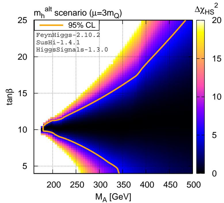
Combining the CMS analysis of  $H, A \rightarrow \tau^+ \tau^-$  with the signal strength data for the observed Higgs boson yields the following exclusion region for the MSSM Higgs sector in the  $m_h^{\text{alt}}$  scenario with  $\mu = 3M_Q$ :
