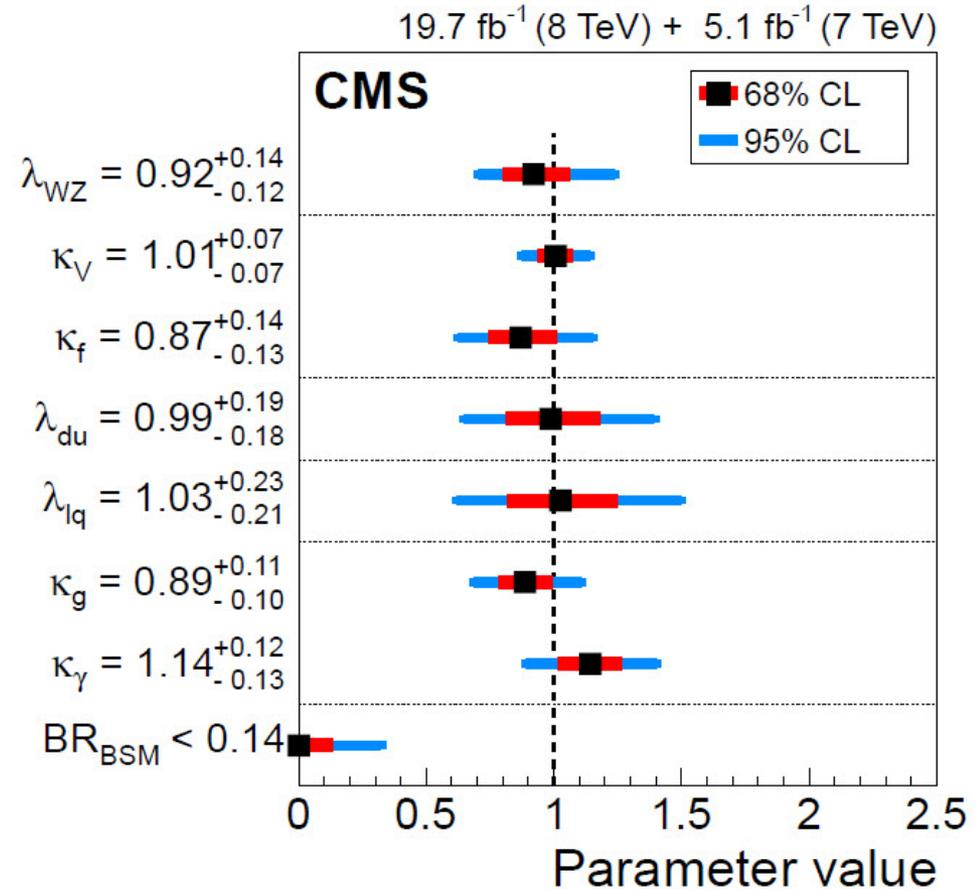
Summary plot of likelihood scan results for the different parameters of interest in benchmark models separated by dotted lines. The  $BR_{BSM}$  value at the bottom is obtained for the model with three parameters  $(\kappa_g, \kappa_\gamma, BR_{BSM})$ . The inner bars represent the 68% CL confidence intervals while the outer bars represent the 95% CL confidence intervals. Taken from arXiv:1412.8662 (December, 2014).
