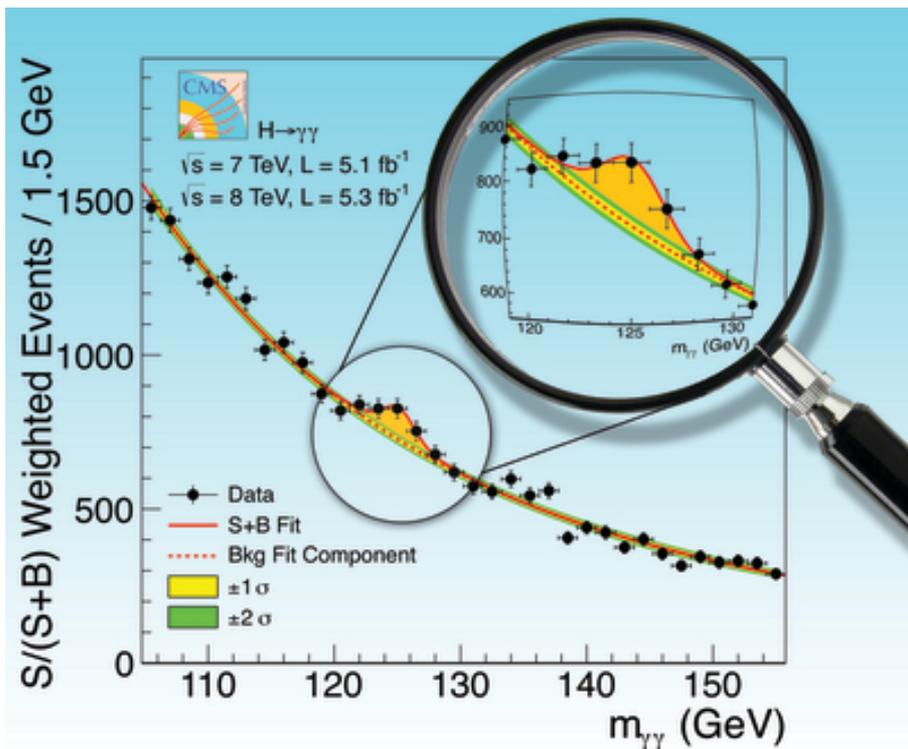
The diphoton invariant mass distribution with each event weighted by the  $S/(S+B)$  value of its category. The lines represent the fitted background and signal, and the colored bands represent the  $\pm 1$  and  $\pm 2$  standard deviation uncertainties in the background estimate. The inset shows the central part of the unweighted invariant mass distribution. Taken from Physics Letters **B716** (2012) 30—61.
