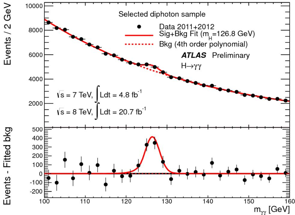
Invariant mass distribution of diphoton candidates for the combined 7 TeV and 8 TeV data samples. The result of a fit to the data of the sum of a signal component fixed to  $m_H = 126.8$  GeV and a background component described by a fourth-order Bernstein polynomial is superimposed. The bottom inset displays the residuals of the data with respect to the fitted background component. Taken from ATLAS-CONF-2013-012 (March, 2013).
