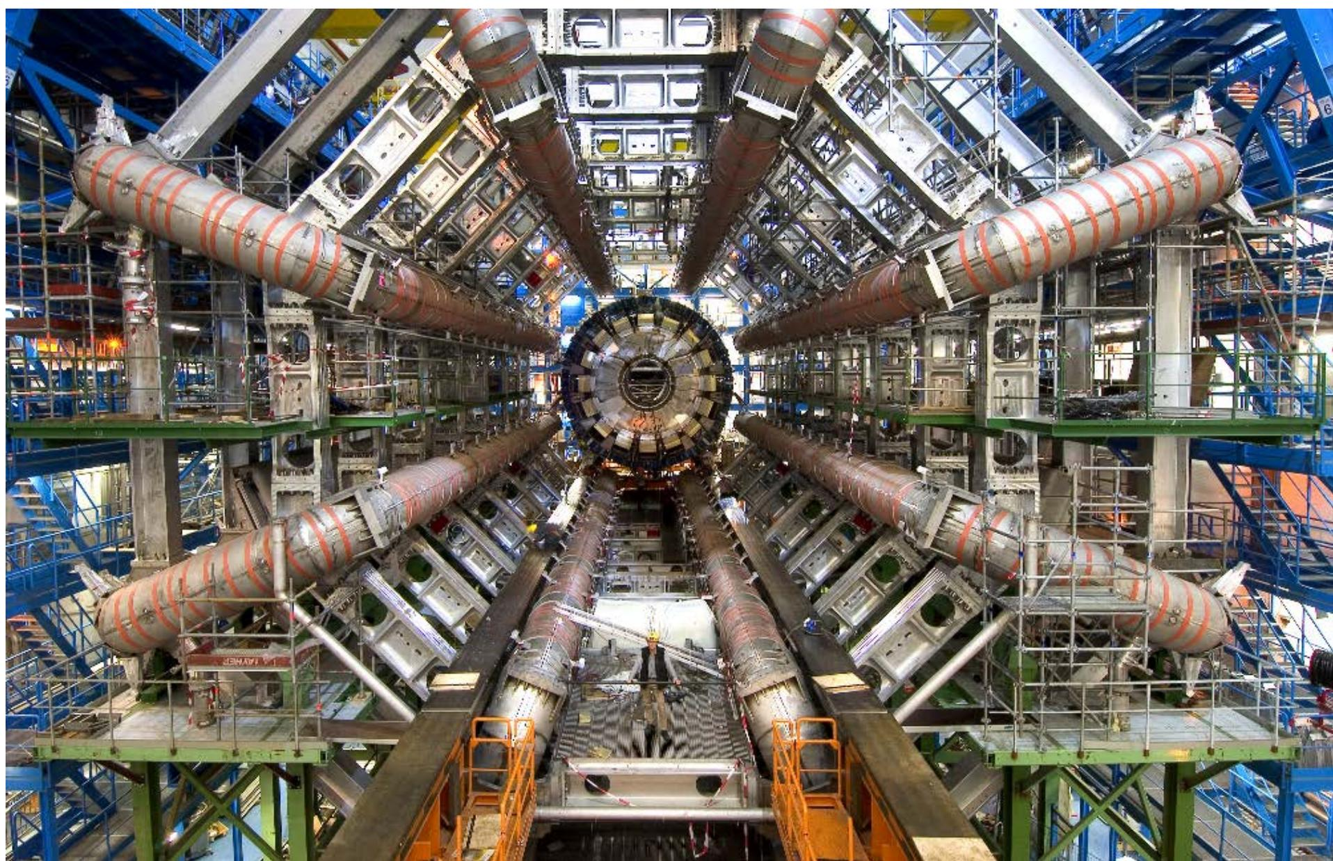
Different elements of the detector help to distinguish particles that are produced in the collision.
