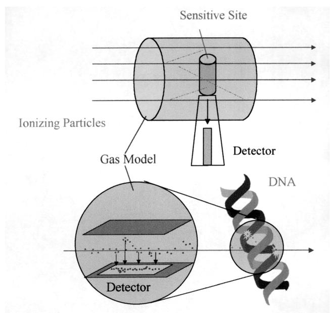
Fig. 1 – Two different approaches to perform nanodosimetry in a low-pressure gas model.
