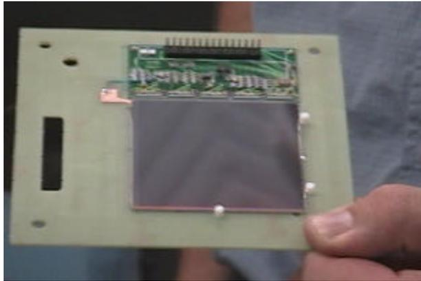
**Fig. 1.** One of the two existing silicon modules. The 6.4cm x 6.4 cm silicon strip detector and the readout electronics are visible.
