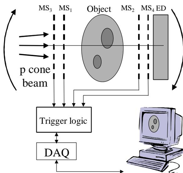
**Fig. 3.** Conceptual approach to proton computed tomography. MS = silicon microstrip detector; DAQ = data acquisition system; ED = energy detector
