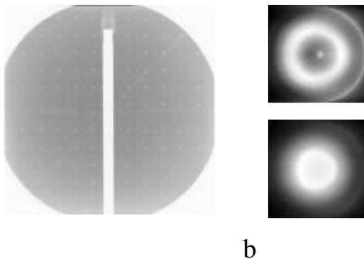
**Fig. 2.** (a) Digital x-ray radiograph of a cylindrical test object taken with on one of the LLUMC proton gantries. (b) Reconstruction of two tomographic images showing cross-sectional views of the object.
