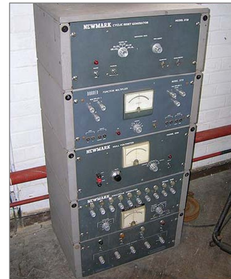
A 1960 Newmark analog computer, made up of five units. This computer was used to solve differential equations and is currently housed at the Cambridge Museum of Technology (from Wikipedia).
