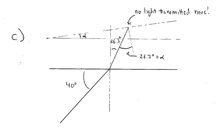
For no light to be transmitted, 26.3°+2 = 0c where Oc is the critical angle, given by
