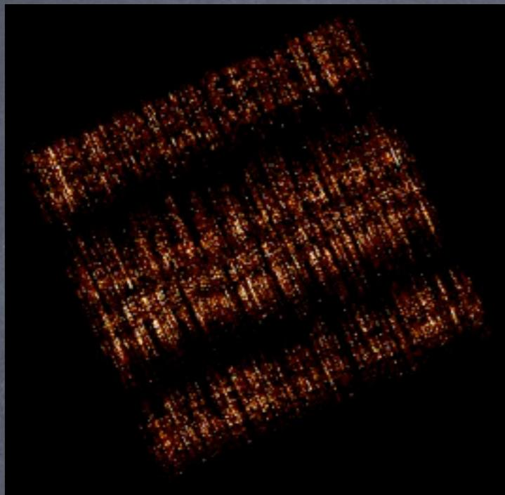
Caused by an error in the serial readout which randomly adds charge to columns as they are read out. Effects a small fraction of frames for any given column, and a software routine exists to remove them. Image shows only events identified as streaks.
