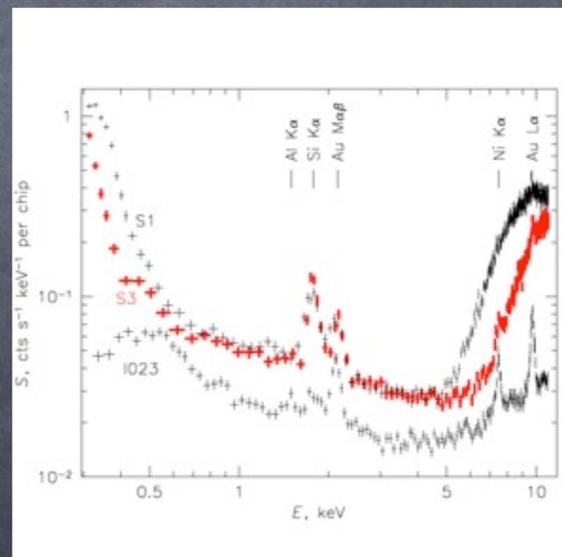
Line features are due to fluorescence of material in the telescope and focal plane.
