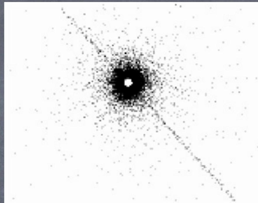
For bright sources both pileup and a readout streak appear. The CCD takes data while it is being readout, so if events occur during readout they appear in the wrong place. **Chandra POG:** "Trailed image of a strong X-ray source. The core of the image is faint due to pileup. Most events here are rejected because of bad grades."
